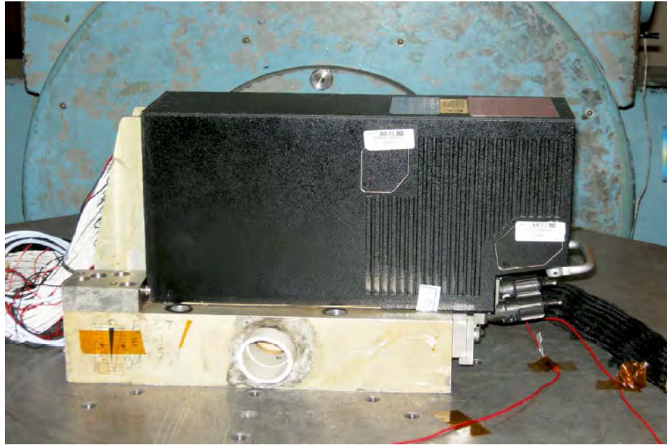
Figure E4: ADIRU undergoing EMI susceptibility testing
