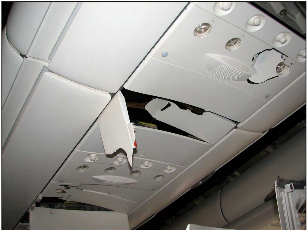
Figure 49: Example of damage to the fittings above passenger seats (rear section)
